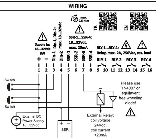
**WARNING:** If a relay will be driven by using an SSR output, supply voltage of device and the coil voltage of relay should be 24Vdc, and coil current should be less than or equal to 20mA. Also a free wheeling diode (1N4007 or compatible) should be connected across the coil terminals as shown at the above figure, otherwise SSR output may damage permanently.
