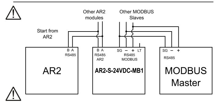
AR2-S-24VDC-MB1 has a selectable internal line termination for MODBUS line for easy commissioning that can be activated easily with en external bridge connection. Please consult to the following documentation for line termination details advised for a MODBUS RS-485 line;
