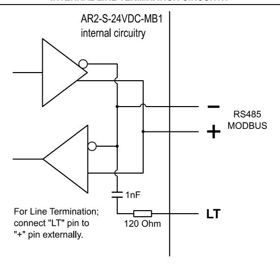
AR2-S-24VDC-MB1 has an internal line termination circuitry for the MODBUS RS-485 line that can be activated easily with an external connection.
